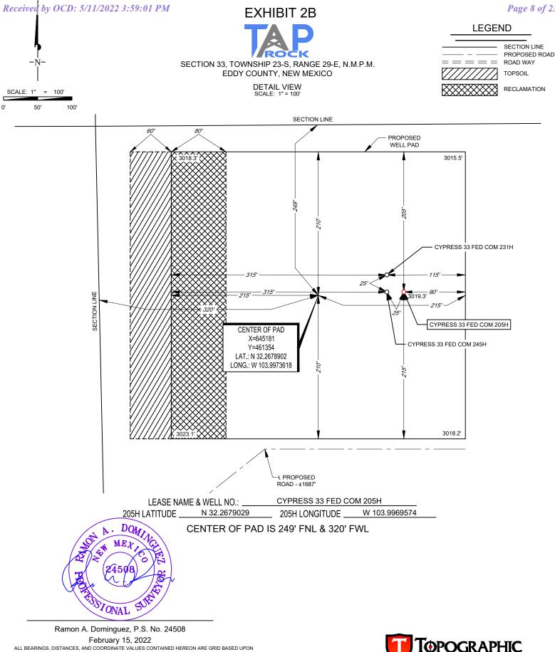
ALL BEARINGS, DISTANCES, AND COORDINATE VALUES CONTAINED HEREON ARE GRID BASED UPON THE NEW MEXICO COORDINATE SYSTEM OF 1983, EAST ZONE, U.S. SURVEY FEET. ELEVATIONS USED ARE NAVD88, OBTAINED THROUGH AN OPUS SOLUTION.
