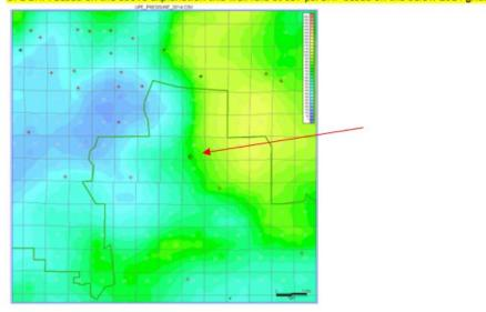
MV BHP: Based on the above explanation this well falls at 1135 psi BHP based on the below 2011 grid.
