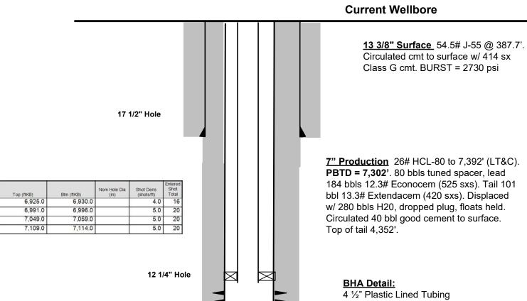
**7" Production** 26# HCL-80 to 7,392' (LT&C). PBTD = 7,302'. 80 bbls tuned spacer, lead 184 bbls 12.3# Econocem (525 sxs). Tail 101 bbl 13.3# Extendacem (420 sxs). Displaced
