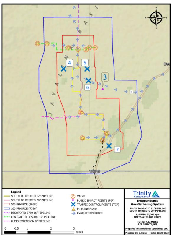
Figure 6: South system to Desoto (12" pipeline) system map
