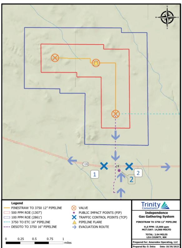
Figure 2: Pinestraw to 3750 (12" pipeline) System Map
