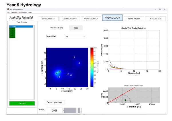
Year 5 Probabilistic Hydrology (note no crossover between blue delta-press. & green fault slip press.)
