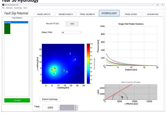
Year 30 Probabilistic Hydrology (note no crossover between blue delta-press. & green fault slip press.) Fault Slip Potential v1.07
