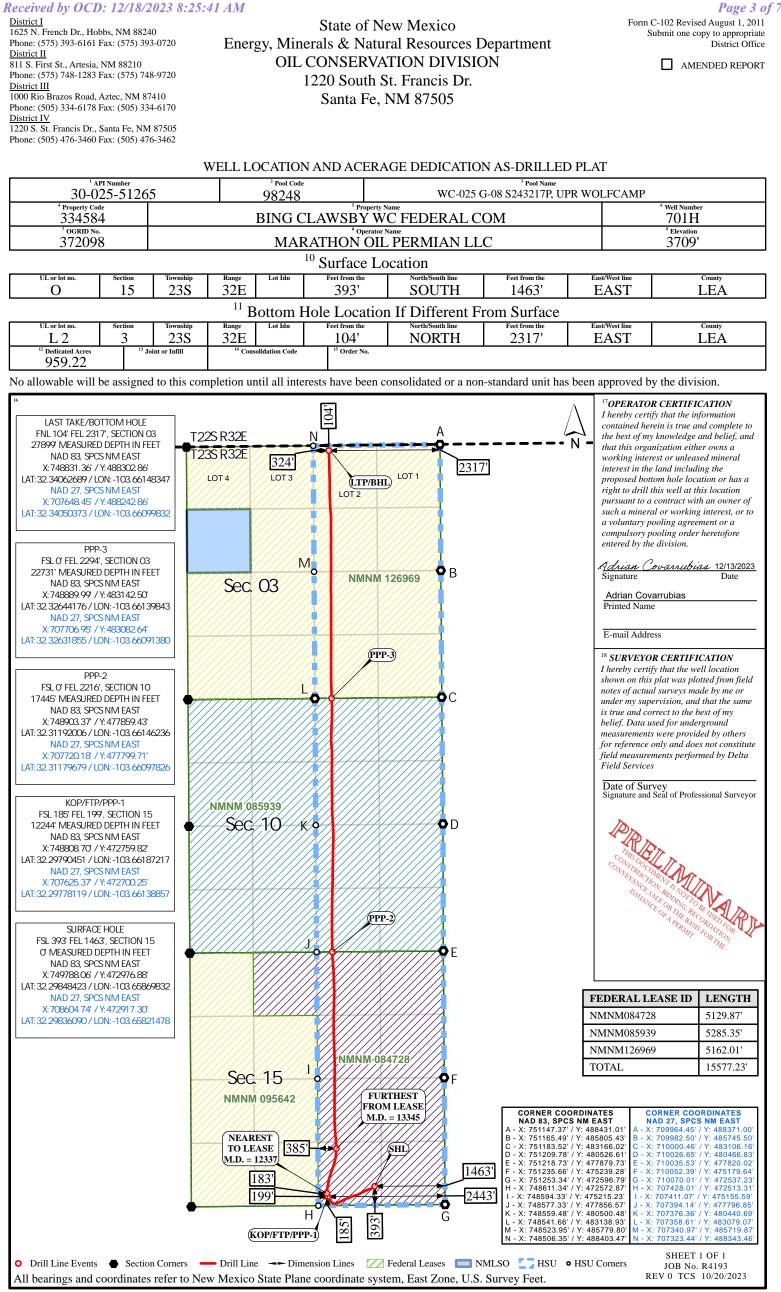
Distances/areas relative to NAD 83 grid measurements. Combined Scale Factor: 0.99914426 and a Convergence Angle: 0.12164755° *Released to Imaging: 12/28/2023 3:06:05 PM*
