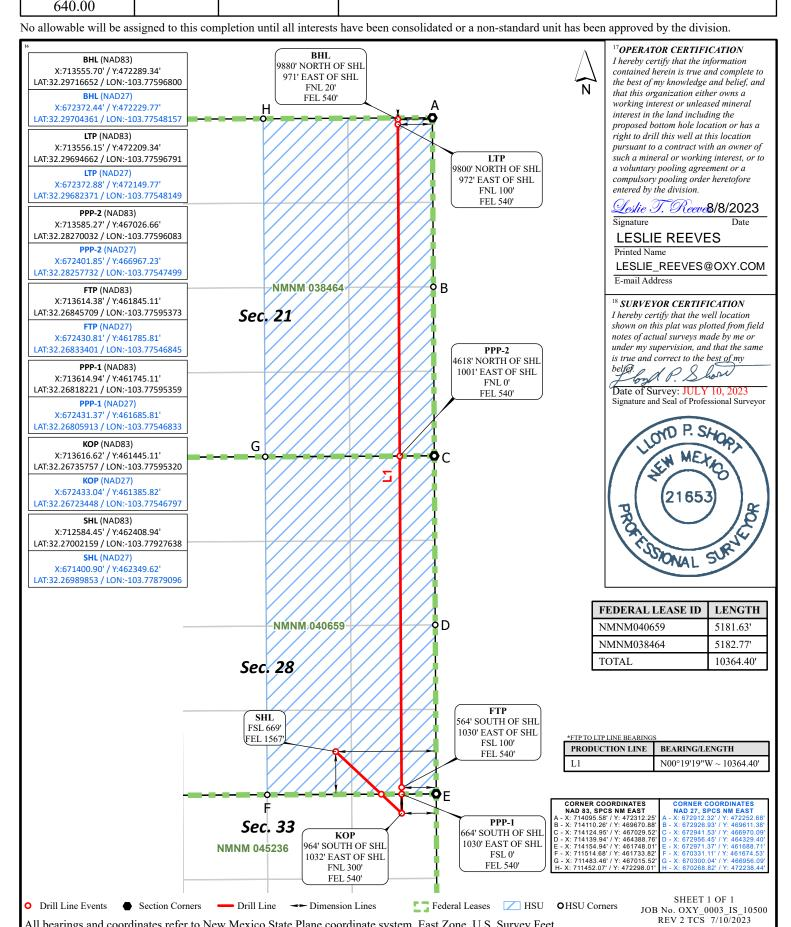
All bearings and coordinates refer to New Mexico State Plane coordinate system, East Zone, U.S. Survey Feet.
