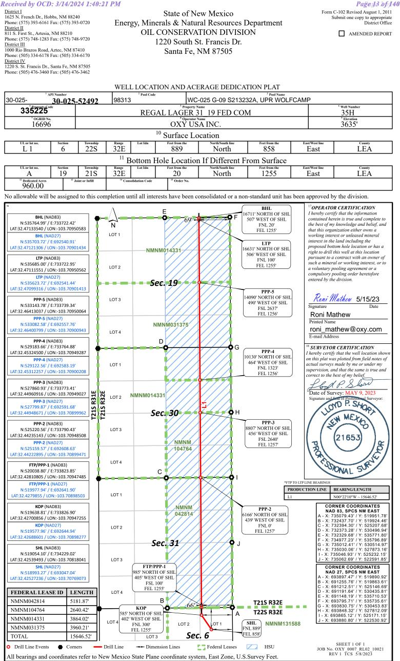
All bearings and coordinates refer to New Mexico State Plane coordinate system, East Zone, U.S.Survey Fe Distances/areas relative to NAD 83 Combined Scale Factor: 0.99977642 Convergence Angle: 00°19'39.03' *Released to Imaging: 5/30/2024 5:05:31 PM*
