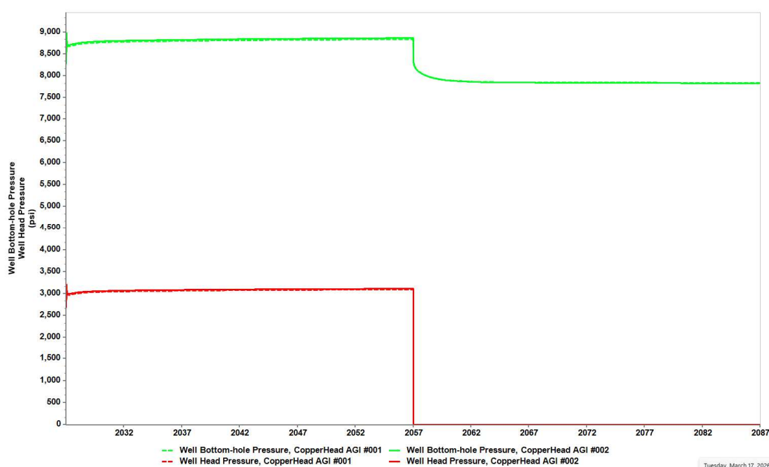
Figure IV-6 Bottom hole pressure and wellhead pressure of Copperhead AGI #001 and #002 at 26 MMSCFD critical pressure Front
