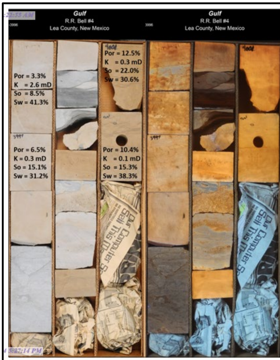
Exhibit L-11: One of the key indicators of an ROZ, the staining of the core with oil over the San Andres is strong used to Image: 2/13/2025 7:08:50 PM
