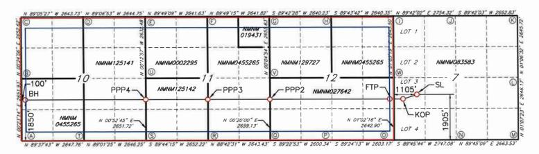
GEODETIC\_DATA NAD 83 GRID - NM EAST <u>SURFACE LOCATION (SL)</u> N: 576930.9 - E: 575499.2 LAT: 32.5859880" N LONG: 104.2224188" N W
