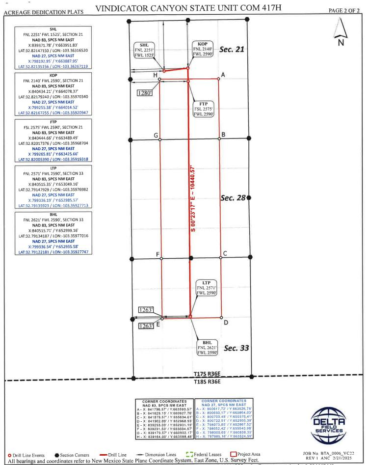
Distances/areas relative to NAD 83 grid measurements. Combined Scale Factor: 0.99981955 and a Convergence Angle: 0.50466944°
