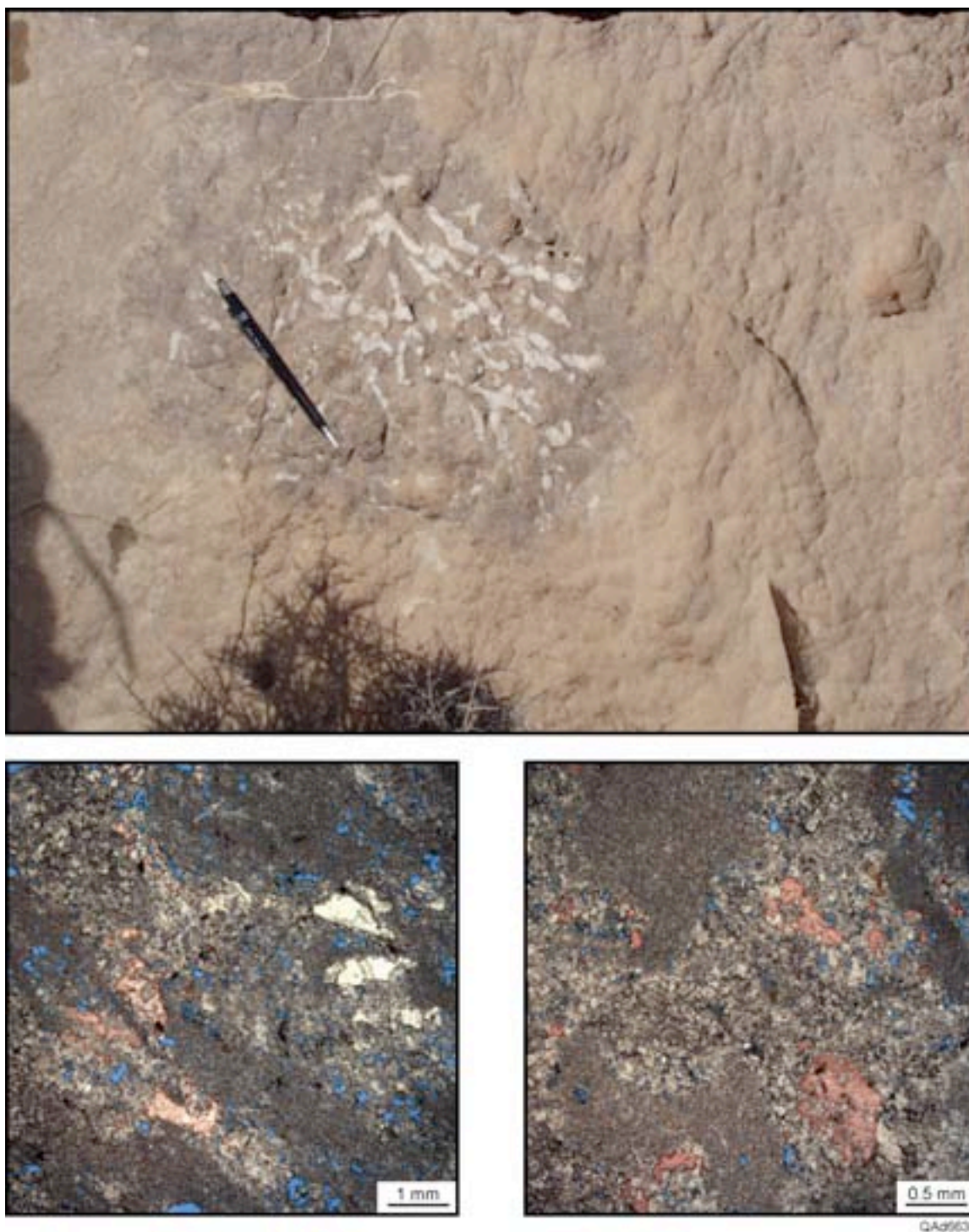
Figure 16. Outcrop photo and corresponding thin section photomicrographs of the Aleman Formation medial bryozoan-rich skeletal packstone, McKelligon Canyon, Franklin Mountains, El Paso, Texas. Note presence of bryozoans both on surface of outcrop and in thin section. Late calcite (stained pink with Alizarin red) partially fills bryozoan molds, but some porosity has been preserved.
