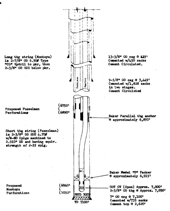
NOTE: DRAWING NOT TO SCALE PROPOSED MECHANICAL INSTALLATION
