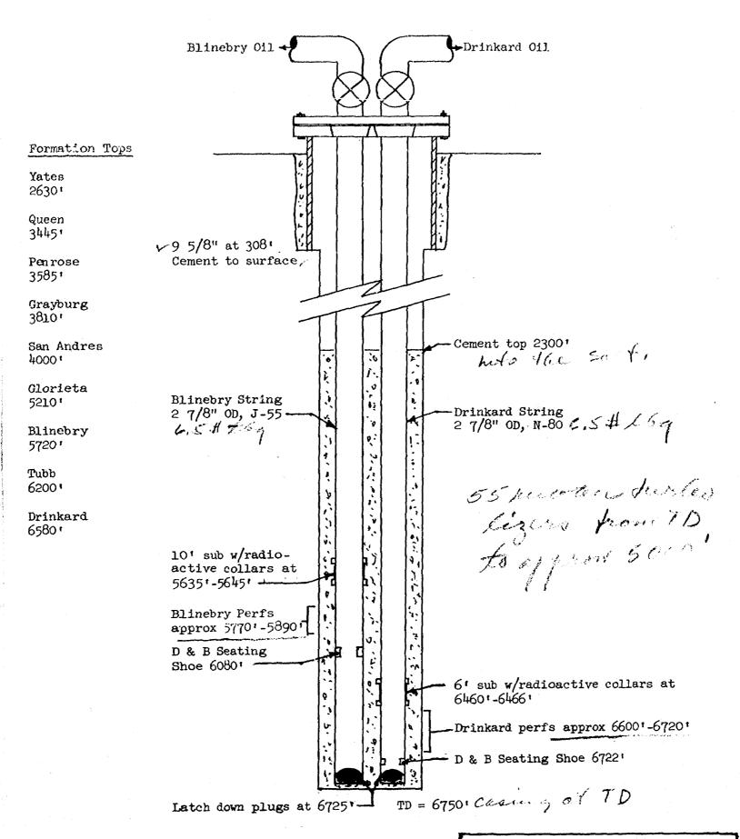
Note: Both strings will be equipped with 55 turbolizers from TD back to 5000
