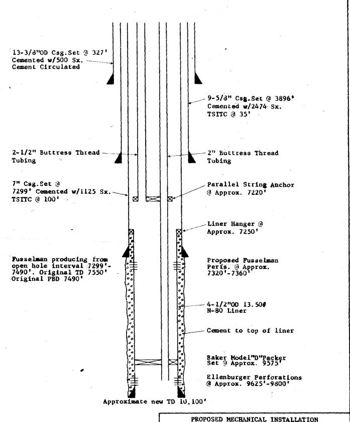
PROPOSED MECHANICAL INSTALLATION DUAL COMPLETION LILLIE WELL NO. 3
