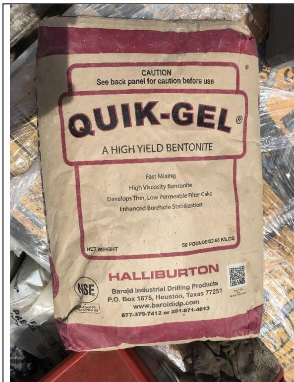
Photo 58—Well grout bentonite amendment.
