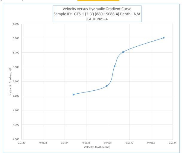
PHYSICAL PROPERTIES DATA - GRANULAR PERMEABILITY (Constant Head Method) - ASTM D2434
