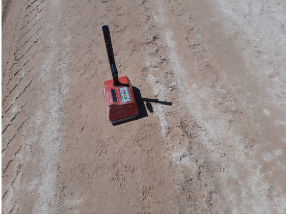
Filename: 20220405_113323 Taking a density test on the east berm of Cell E1
