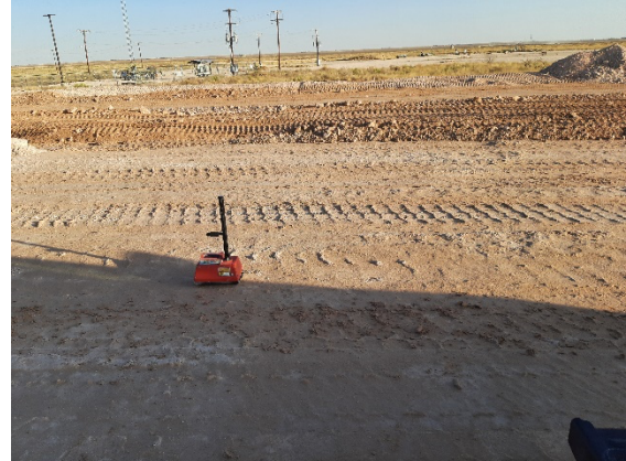
Filename: 20220404_073648 Taking a density test on the north berm of Cell E1
