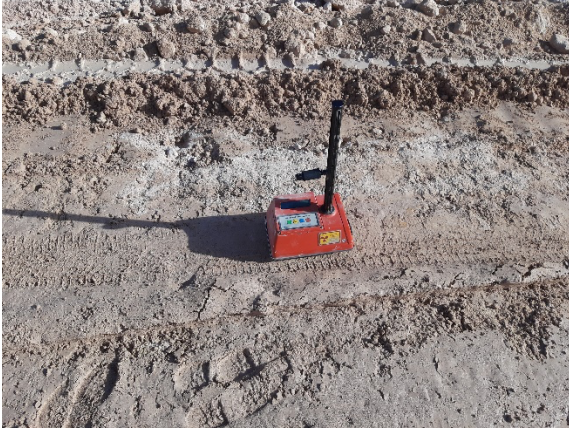
Filename: 20220407_171141 Taking a density test in the north berm of Cell E1
