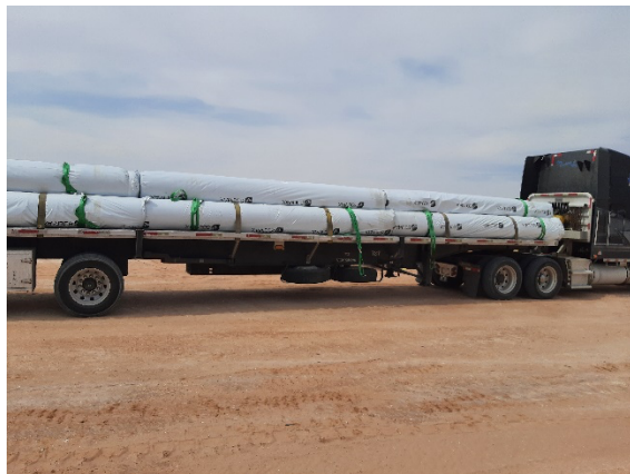
Filename: 20220419_113126 Truck containing GCL being offloaded south of Cell E1
