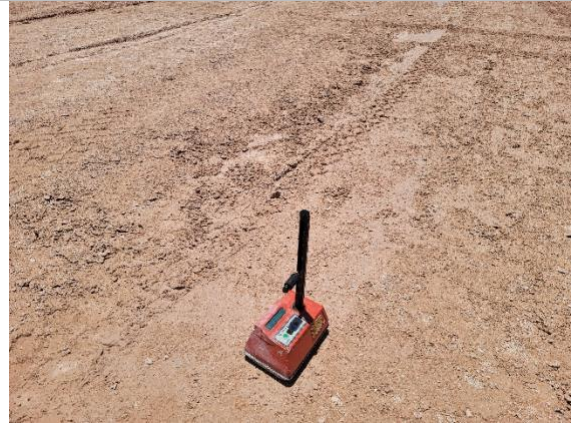
Filename: 20220606_123055 Taking a density test in the Caliche Road west of the west drying pad
