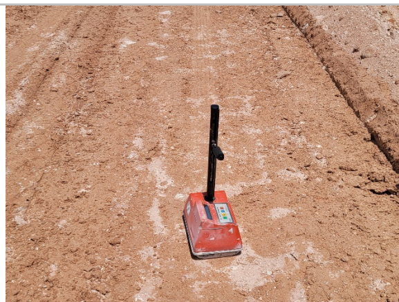
Filename: 20220503_124841 Density test being taken in the west berm
