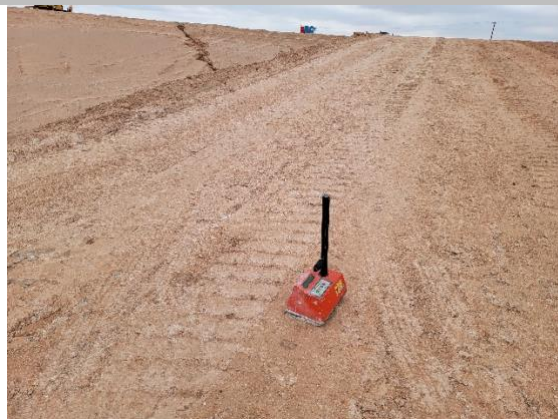
Filename: 20220602_122552 Density testing a lift in the center of the cell ramp
