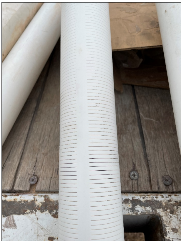
2-inch Sch-40 PVC FJ well screen, 0.010 slot.
