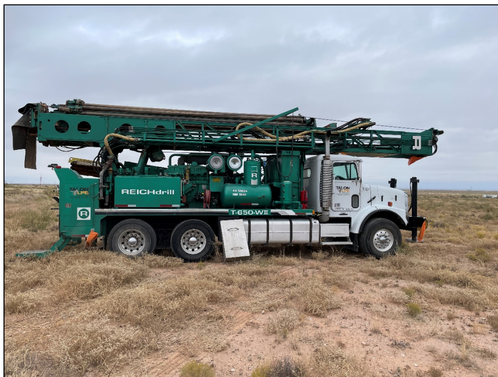
ReichDrill 650-WII air rotary drill rig for well installations.
