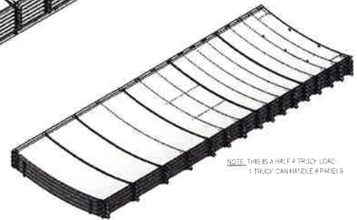
ISOMETRIC VIEW 4 LOOSE TYPICAL PANELS TO BE SHIPPED IN ONE TRUCK SCALE 1:70
