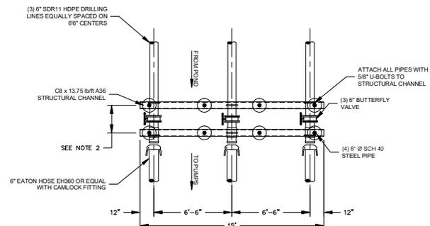
DETAIL 4 - PIPE STAND PLAN VIEW DRILLING
