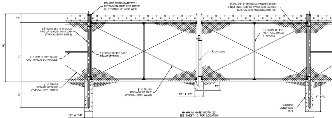
DETAIL 2 - TYPICAL ACCESS GATE DETAIL
