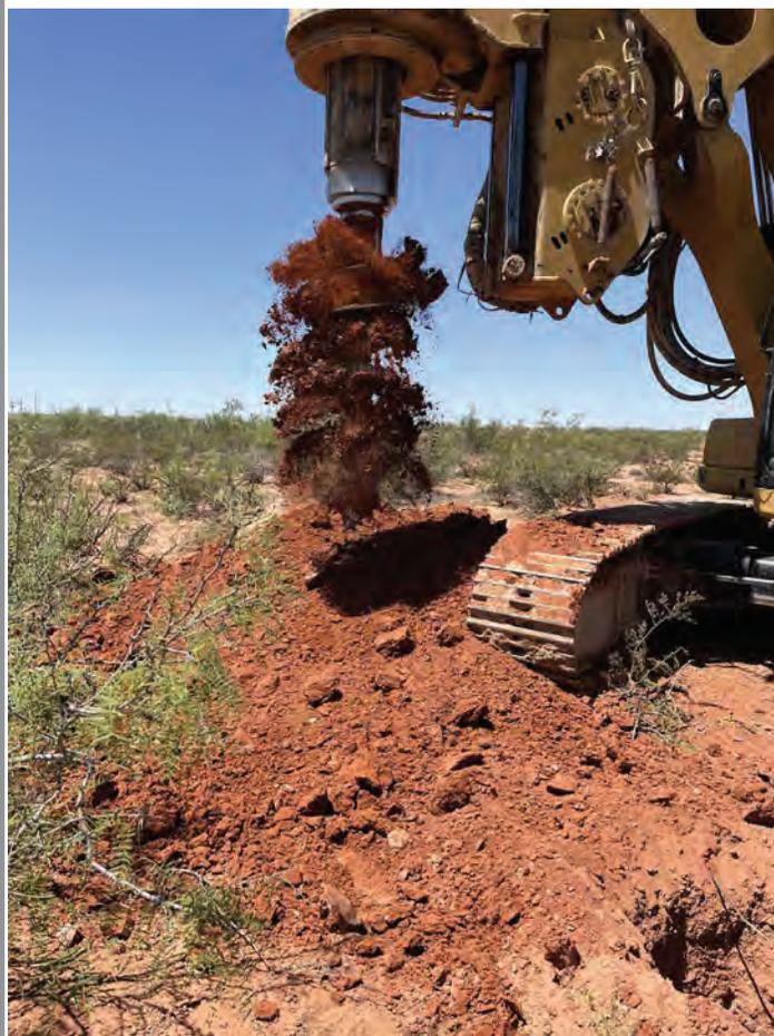
*Due to the lack of groundwater data in the area, Solaris elected to drill an auger boring to 75 feet. This auger spin from total depth (74.33 feet) testifies to the dry boring.*
