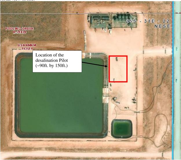
The pilot plant will be in containment by the NE corner of the pond. No new pad location will need to be built for the site.
