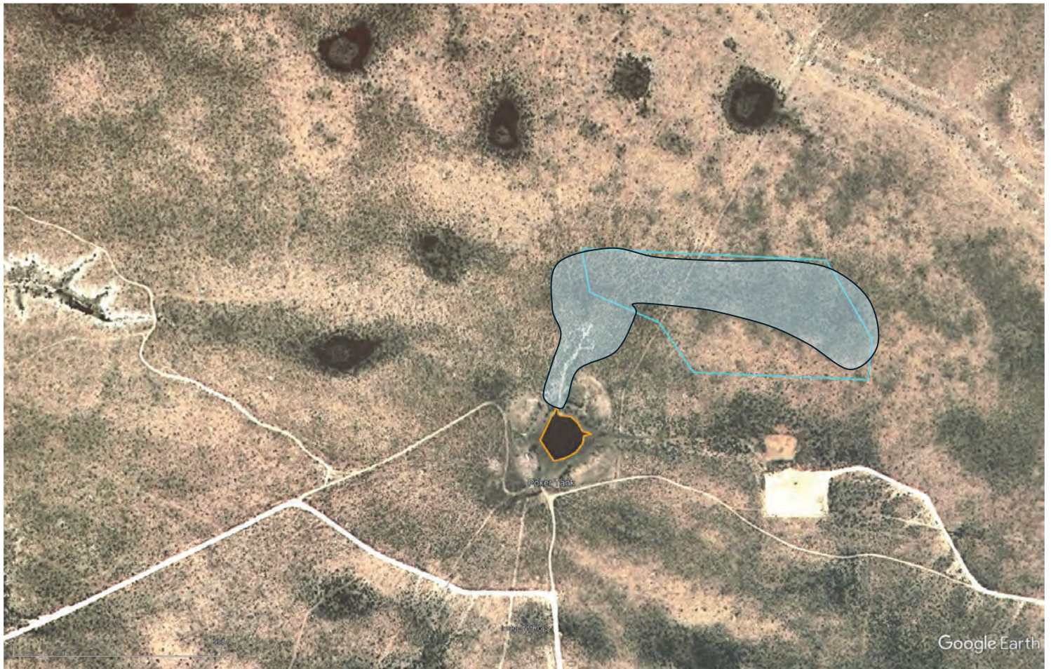
Figure 1 – Google Earth image dated 6/30/2005 showing the maximum water level observed in Poker Tank. The northern swale extension of Poker Tank shown in Appendix Site Photos captured a relatively large drainage area at this time. Low areas in this image are defined by darker vegetation, thus we contend that the area shown in blue likely drained into Poker Tank.
