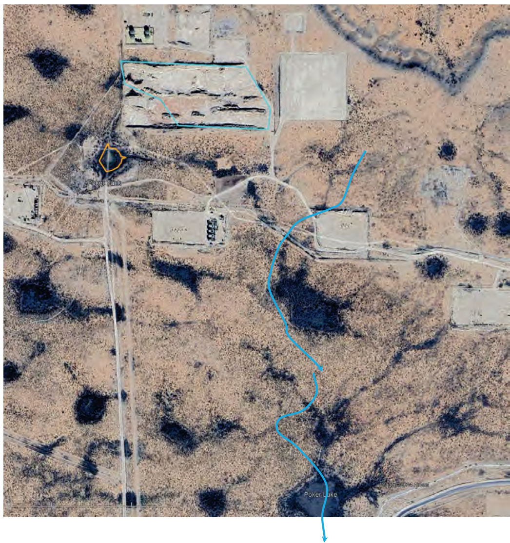
Figure 3 – Probable stormwater flow path east of Mad Cow containment. Infrastructure installed after 2017 diverts stormwater from potentially flowing into Poker Tank to Poker Lake. This is a reasonable conclusion, but without the benefit of a field walk through.
