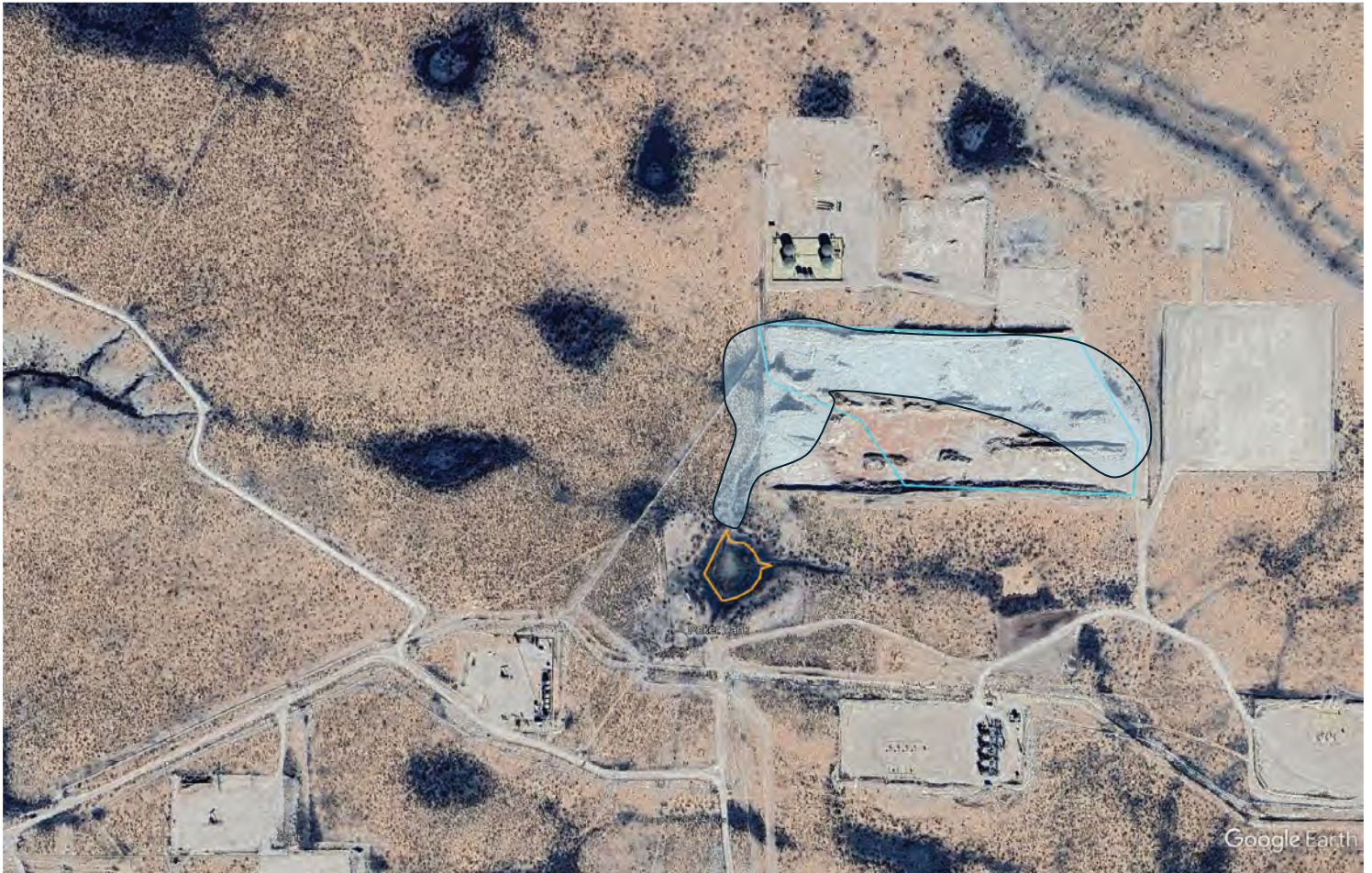
Figure 2- This Google Earth image from 12/31/2024 shows that most of the drainage area of the northern swale into Poker Tank shown in Figure 1 is captured by the caliche quarry. Close examination of this image shows evidence that surface water flow from the area east of the proposed containment, lease roads and the E&P pad flows south to Poker Lake (see Plate 9 and Figure 3) rather than into the east-west swale and into Poker Tank.
