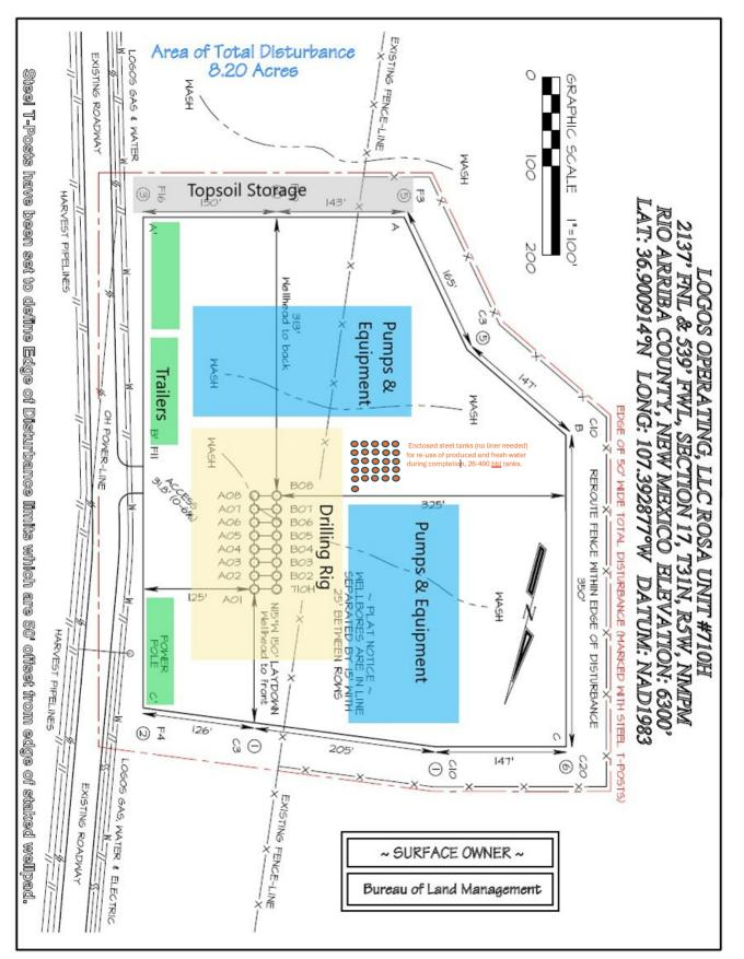
Figure 22. Rosa Unit Pad 26 Proposed Drilling Equipment Layout
