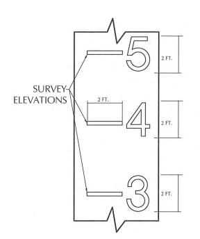
**BERM** NOTE: 1. LEVEL MARKS TO BE LOCATED BY SURVEYOR UNLESS SPECIFIED BY **OWNER BOTTOM OF SUMP**
