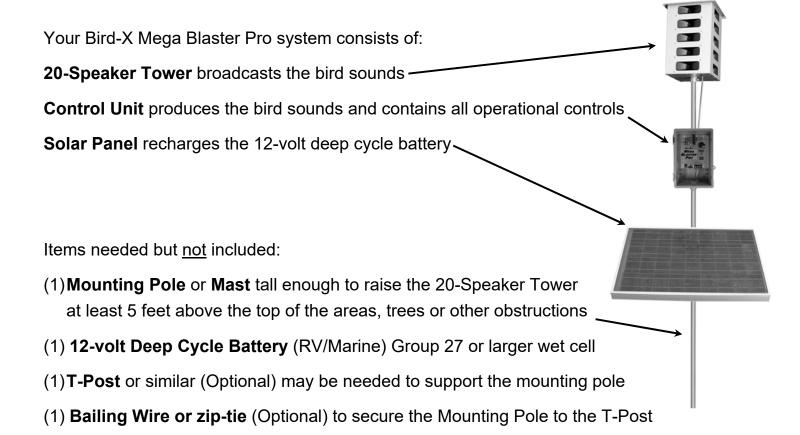
CAUTION: THE MEGA BLASTER PRO IS CAPABLE OF PRODUCING SOUNDS UP TO 125 DECIBELS. PROPER HEARING PROTECTION MUST BE WORN ANYTIME THE UNIT IS TURNED ON.
