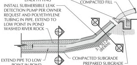
LEAK DETECTION/SAMPLING 6 SYSTEM DETAIL NOT TO SCALE
