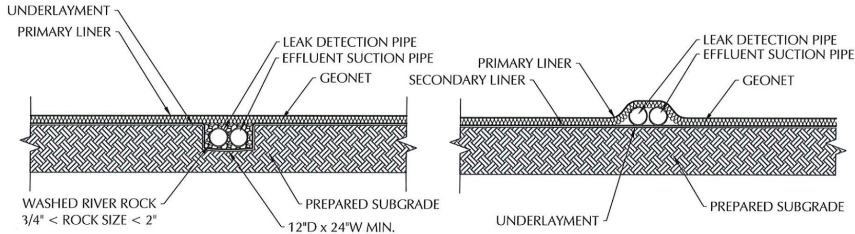
**SUMP LEAK DETECTION PIPE DETAIL** (3)
