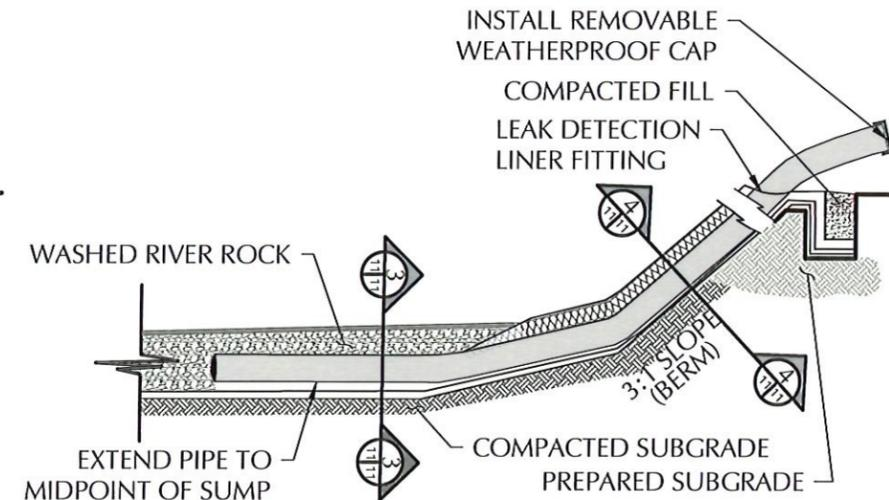
**EFFLUENT SUCTION PIPE SAMPLING SYSTEM DETAIL** (7)
