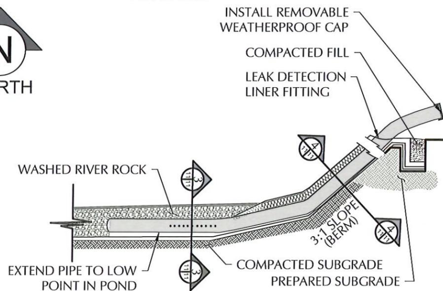
**LEAK DETECTION/SAMPLING SYSTEM DETAIL** (6)
