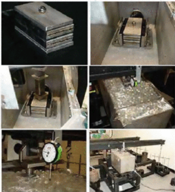
Fig. 2 Compressive environmental stress cracking test equipment
