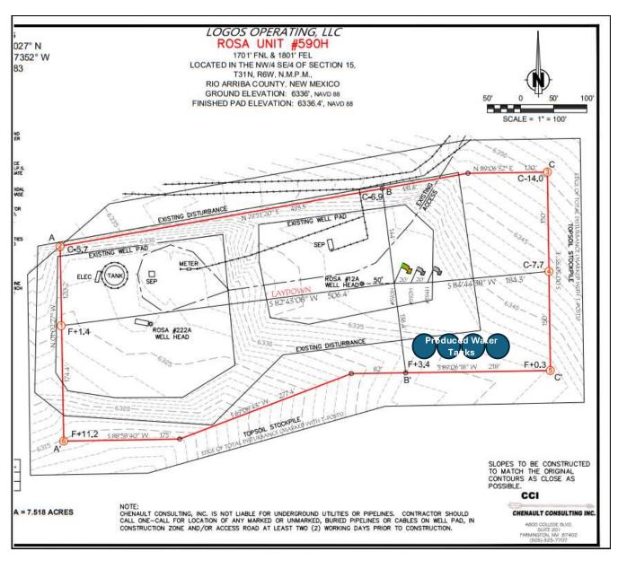
• 3RF-87 - ROSA UNIT 590H API 3003931478, ROSA UNIT 592H API [fVV2512249185] consists of four (4) – enclosed 500 bbl upright tanks with steel walls and steel bottoms.
