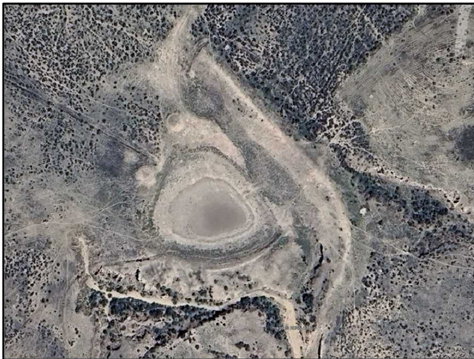
Figure 7. GoogleEarth Imagery Date 5/21/2024 – P03 - evidence of manmade pond; note the dike on the eastern side.
