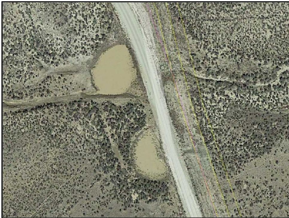
Figure 6. GoogleEarth Imagery Date 10/13/2017 – P01 and P02 - evidence of manmade livestock ponds; note the surrounding dikes constructed to contain water.
