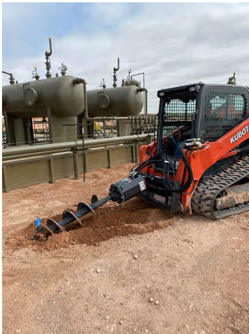
The mechanical auger used to obtain deeper samples on the pad and in the pasture.
