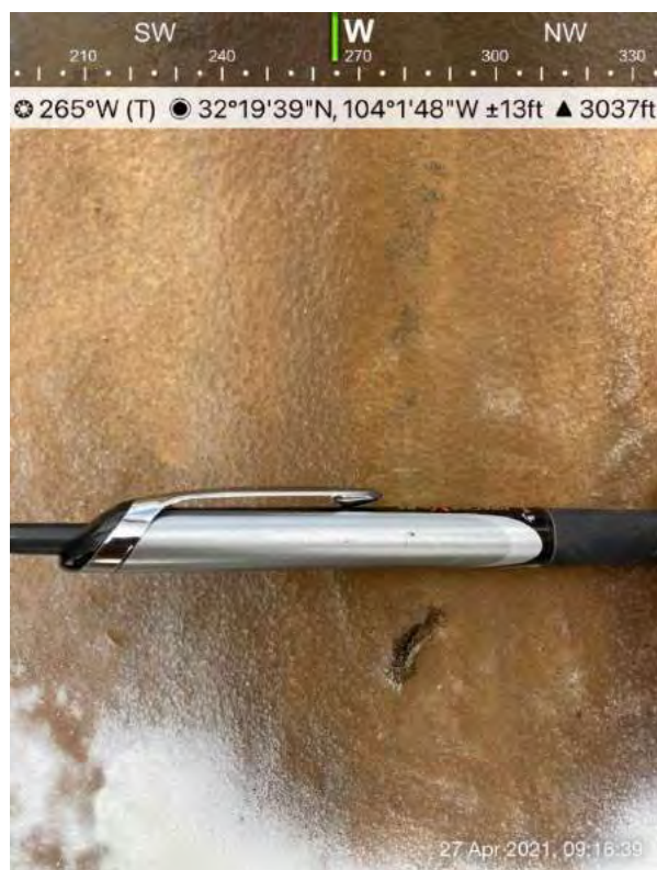
3/4" Diameter Hole North of Tank F55472
