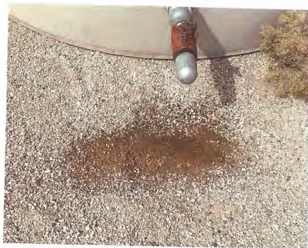
Minor scraping reveals signs of a release.
