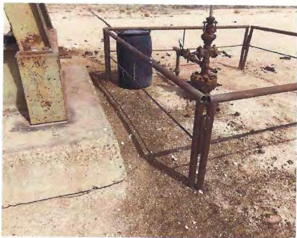
Picture of wellhead. Release radiates out following pumpjack base.
