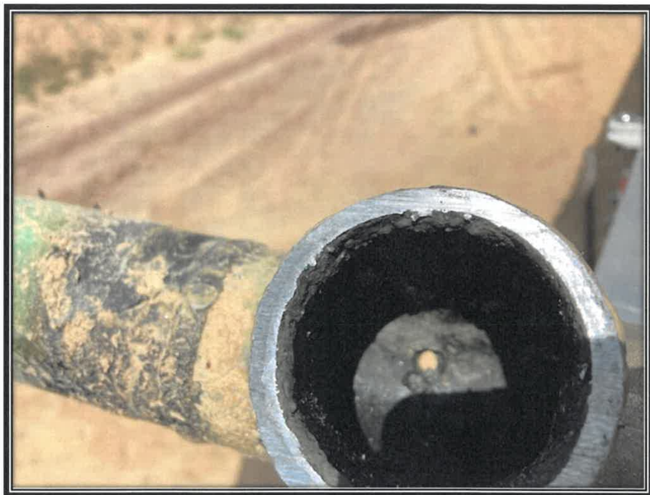
Internal corrosion leak in a two inch tee, part of the water dump line.
