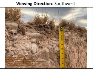
5in of topsoil. East side of excavation.
