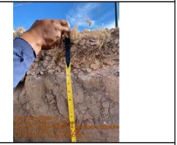
6in of topsoil down to aggregate. South side of excavation.
