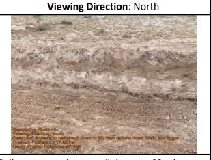
Soil appears to be topsoil down to 2ft, then caliche down to 4ft, and aggregate down to 6ft
