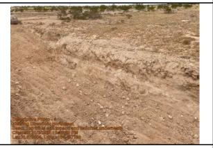
Top 2ft is still topsoil and caliches underneath
