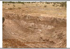
Top 2ft near BES21-01 is topsoil. Below that is caliche.
