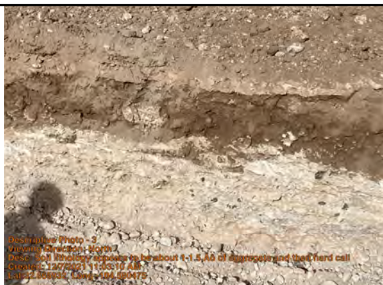
Soil lithology appears to be about 1-1.5' of aggregate and then hard caliche down
