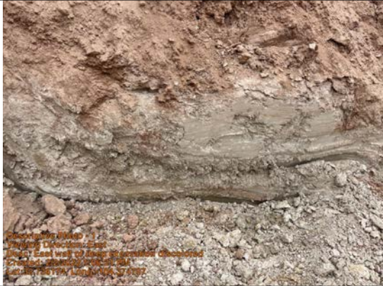
East wall of deep excavation discolored at 18'
