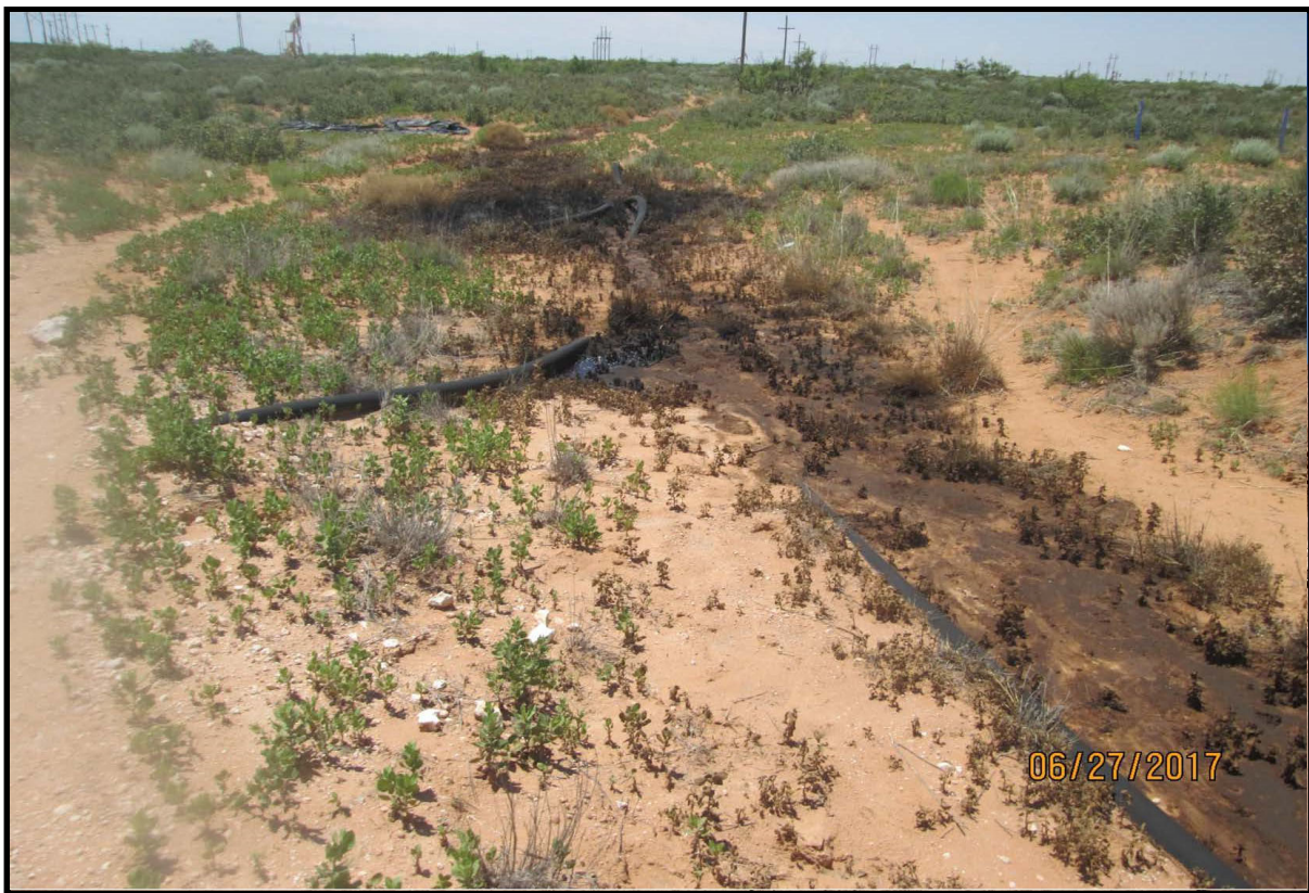
View of the initial release point at the failed poly line (June 27, 2017), facing northwest.
