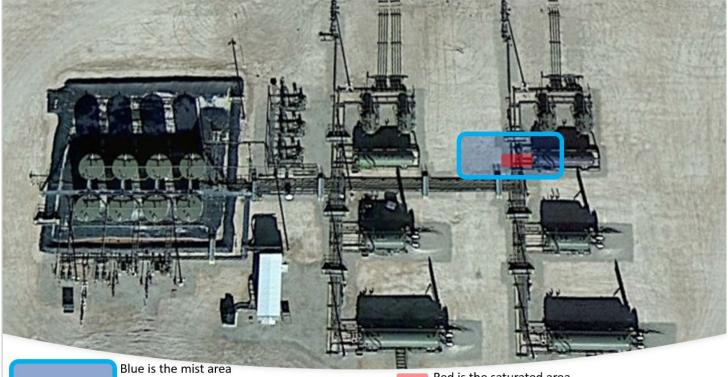
70ft x 50ft x 0.125in x 0.125in (Soil Penetration) Light Blue outline is the total area 90ft x 60ft Red is the saturated area 20ft x 10ft x 1in x 1.25in (Soil Penetration)
