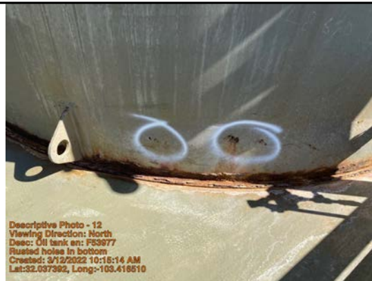
Oil tank sn: F53977 Rusted holes in bottom
