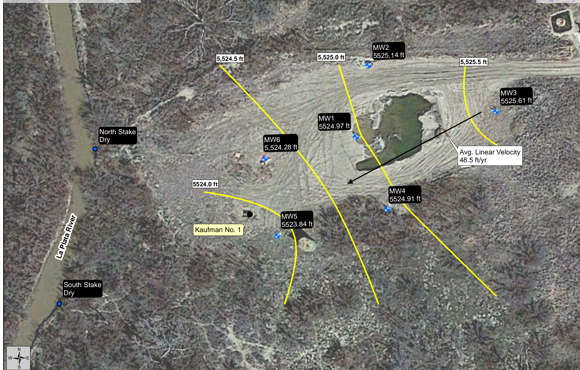
Figure 5 Potentiometric Surface Elevation Map
