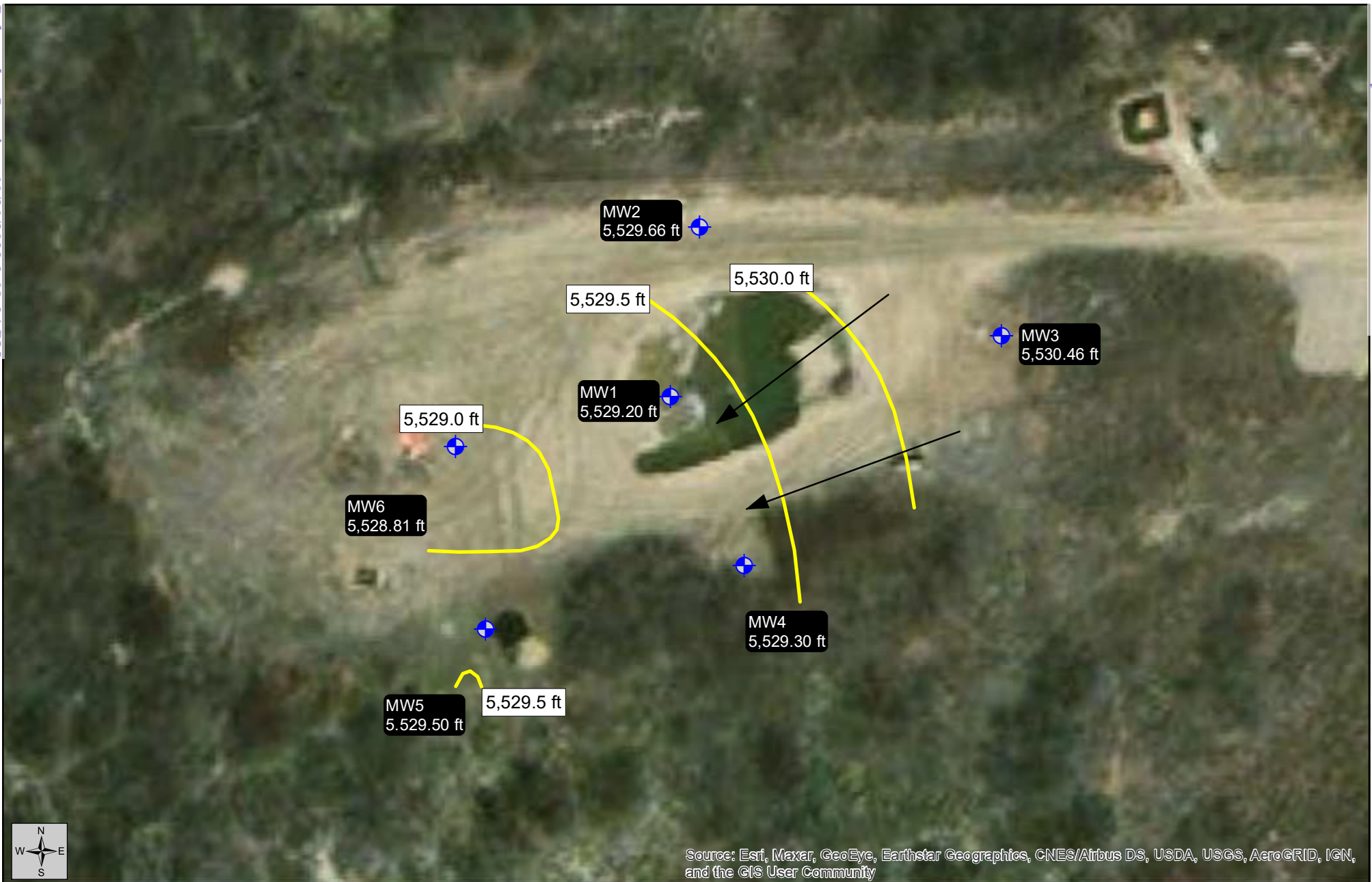
Figure 4 Potentiometric Surface Elevation Map - January 2019
