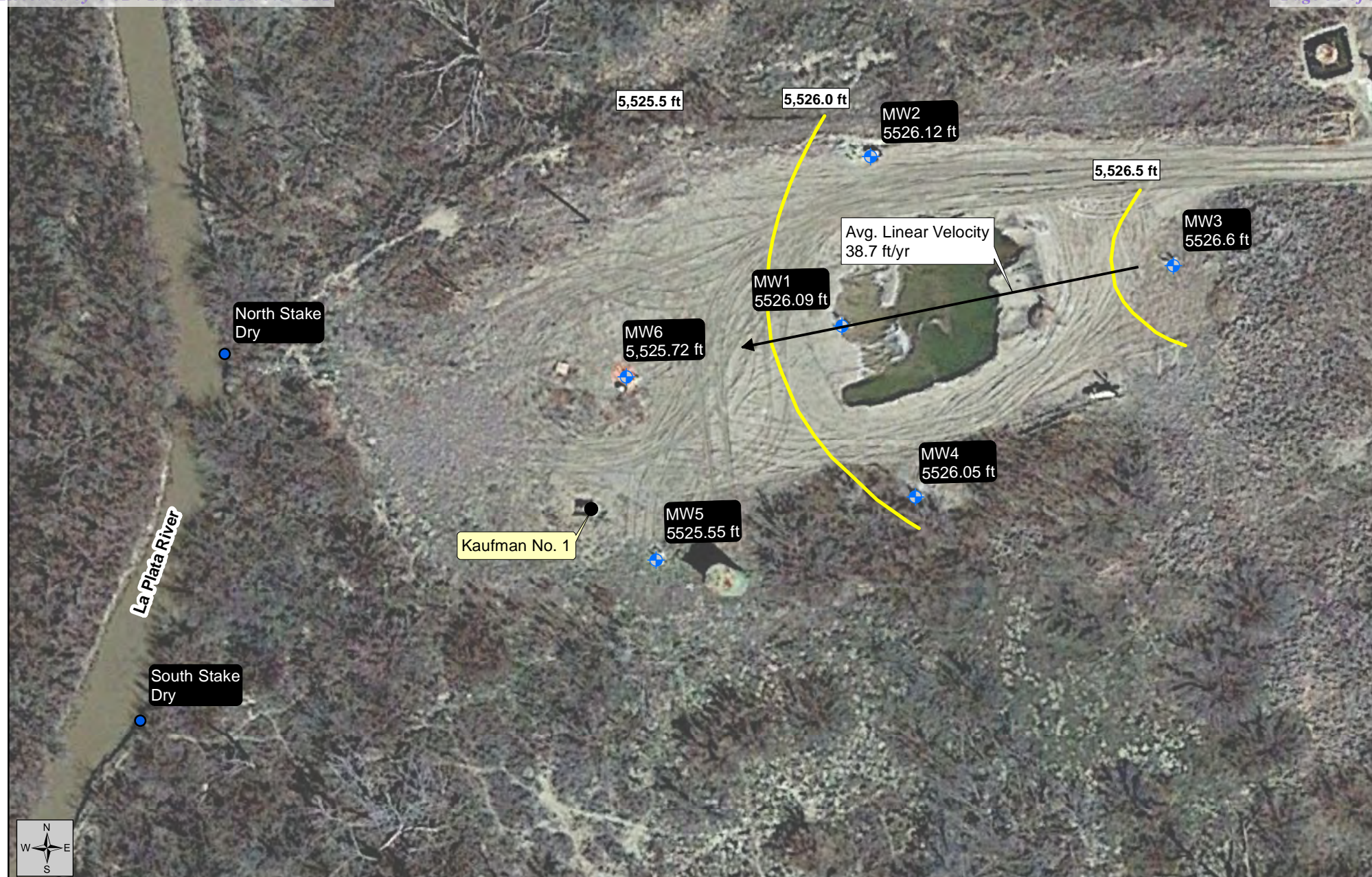
Figure 5 Potentiometric Surface Elevation Map
