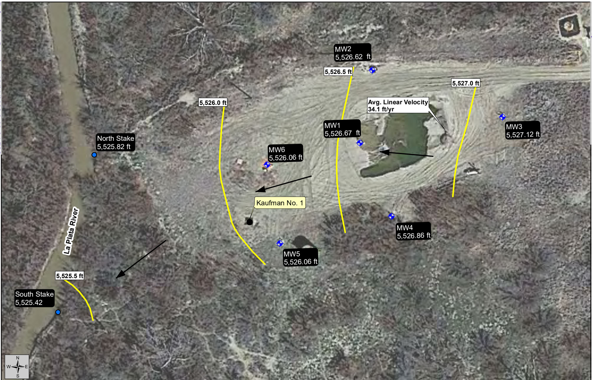
Figure 5 Potentiometric Surface Elevation Map
