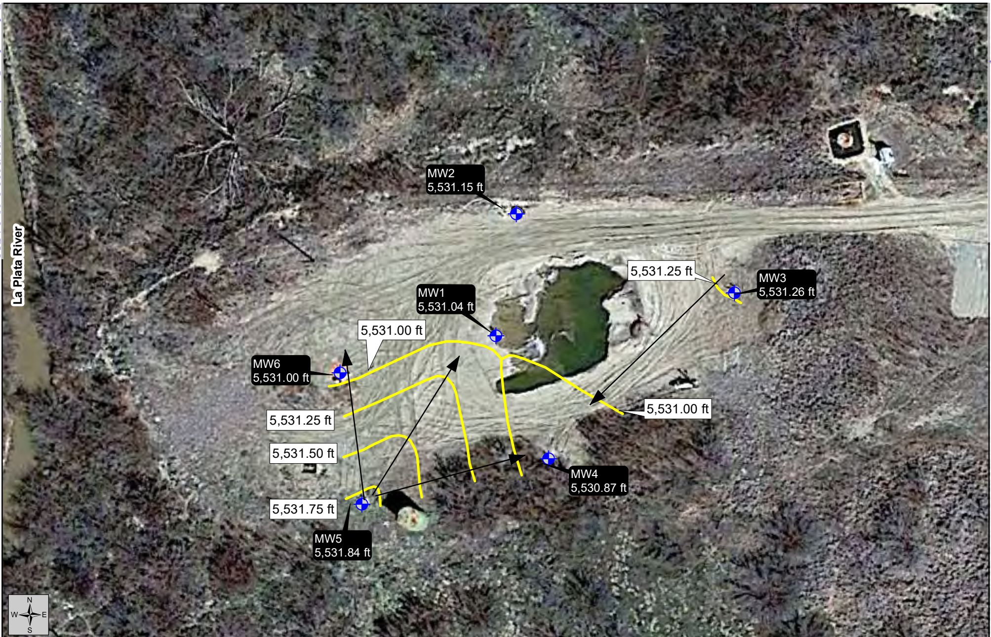
Figure 8 Potentiometric Surface Elevation Map - June 2019
