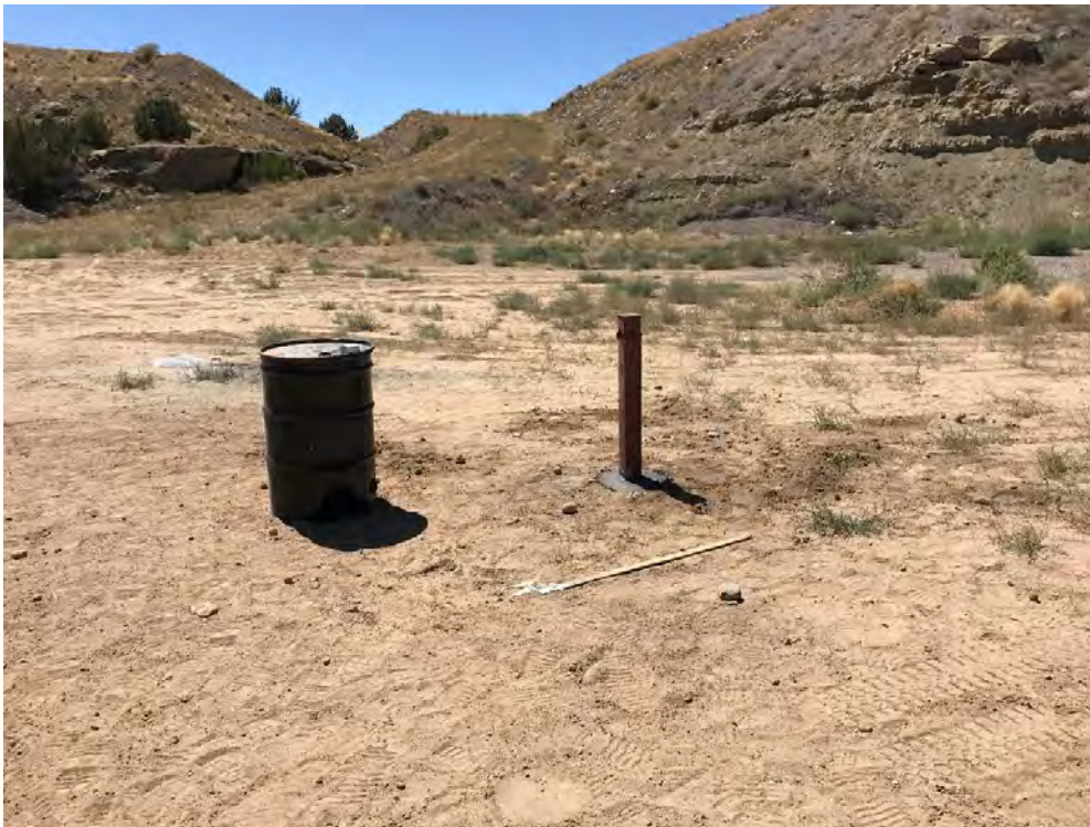
Photograph 8: MW03 completed well, 35 feet.
