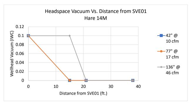
The above figure illustrates that vacuum influence was observed at a distance of 15 feet at 136 IWC at 46 standard cubic feet per minute (scfm). Vacuum response was not observed at 21 feet. Based on the vacuum observations a ROI of 15 to 20 feet can be assumed.
