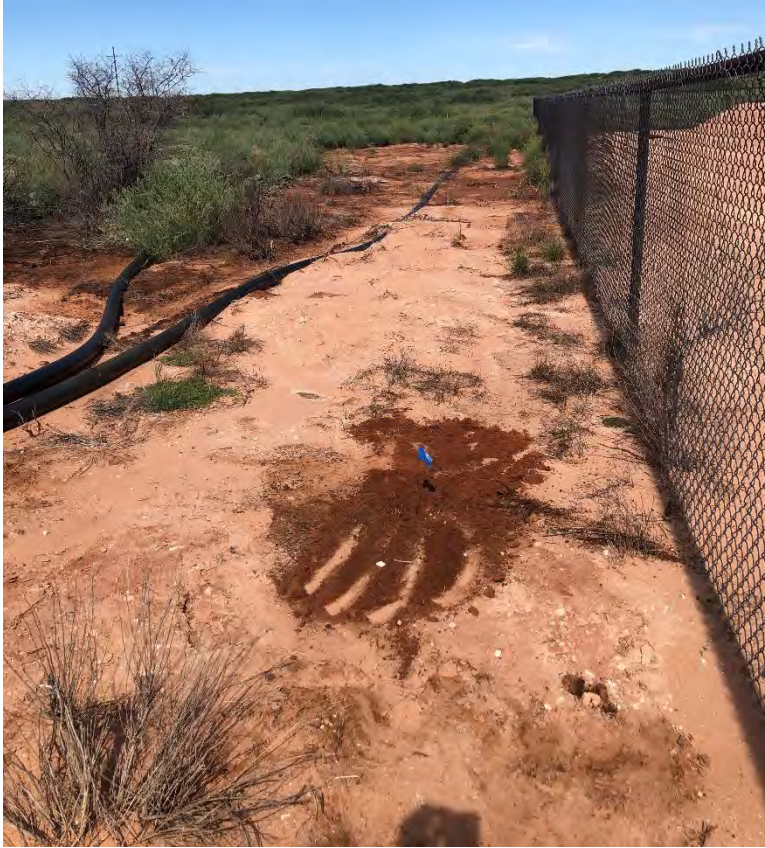
SP5 This 2021 image shows the 2021 sample boring at the same location as the 2020 sample T3. Soil staining and stressed vegetation remains in many areas of the spill footprint while much of the spill footprint is re-vegetated.
