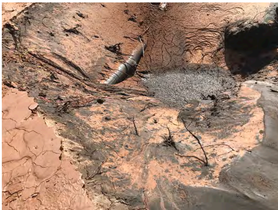
View of point of release – rupture in poly pipe
