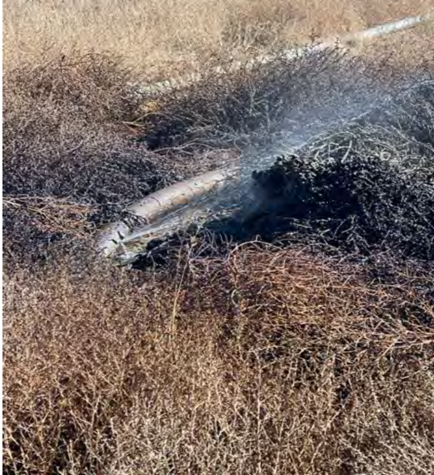
View East – Origin of spill. Cause of the release is due to property damage on associated flowline.
