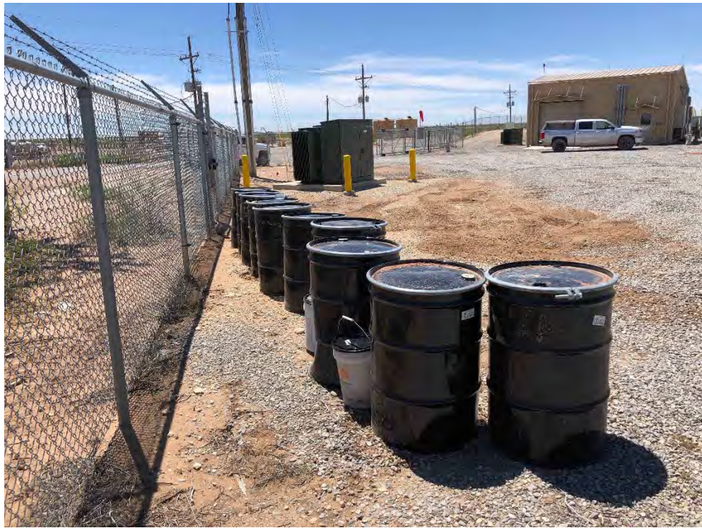
Photo 4: View facing southeast of drummed soil cuttings from SB-East, SB-North, and SB-South. The drums were stored along the northeast fence line of the Artesia Station West yard.
